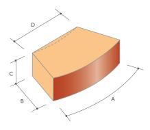
NOTE: Bonding - Note that RD.I and RD.2 types cannot be used together in the same one brick thick wall either in English or Flemish Bonds, to produce ideal alignment of the perpends on the concave face, except when the outside radius exceeds 3m.
