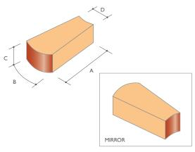
NOTE: Bonding - Note that RD.1 and RD.2 types cannot be used together in the same one brick thick wall either in English or Flemish Bonds, to produce ideal alignment of the perpends on the concave face, except when the outside radius exceeds 3m.
